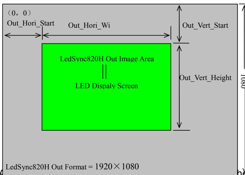
The images in LedSync820H output window for the LED display are defined by the following 4 groups of parameters:
